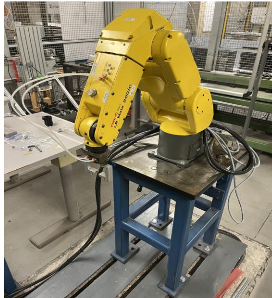
Figure 1: FANUC LR Mate 200iC used as the Target Compact-Industrial-Robot Platform. The Monitoring Method is Implemented as a Controller-Independent Retrofit; Photograph Supplied by the Authors.
