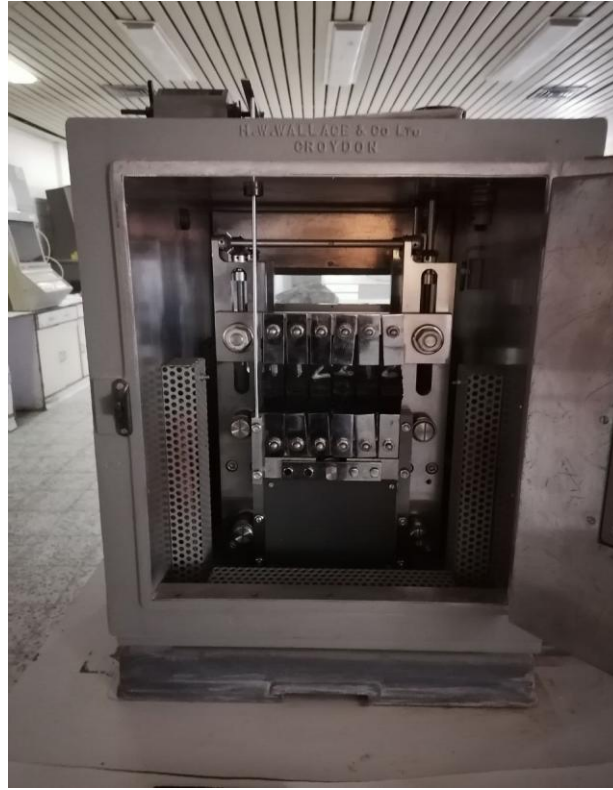
Figure 5: The Fatigue Test Setup
