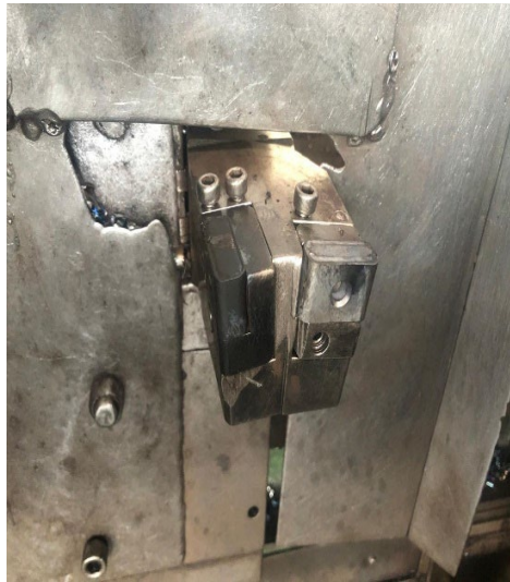
Figure 2: The Proposed Experimental Dual Interchangeable Carbide Insert
