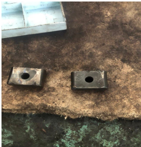
Figure 3. Disassembled Configuration of Dual Carbide Inserts Showing Thermo-Mechanical Effects on the Workpiece Surface
