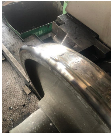
Figure 1: Surface Defects on Wheelsets Leading to Carbide Insert Failure.
