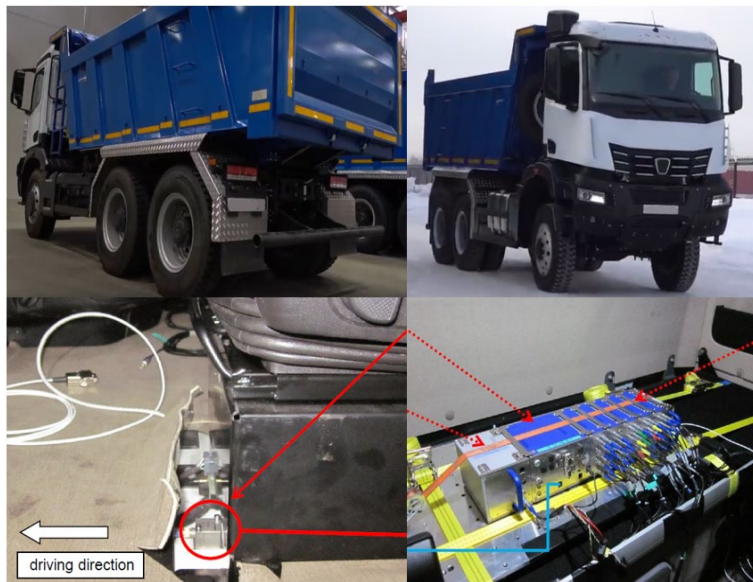
Figure 8: The Experimental Researches of the Triple-axle Dump Truck Smooth Running Characteristics
