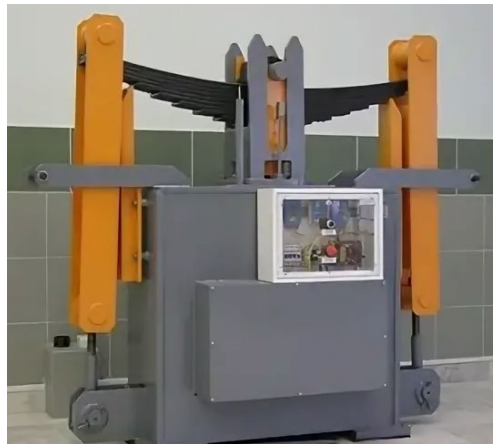
Figure 9: The Vehicle Leaf Springs Bench Tests
