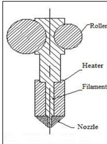
Figure 1. Schematic diagram of a 3D printer extruder
