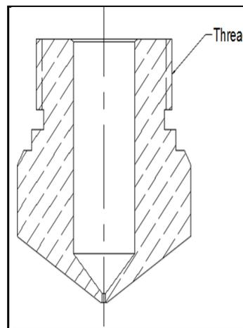
Figure 2. Sectional view of a 3D printer nozzle
