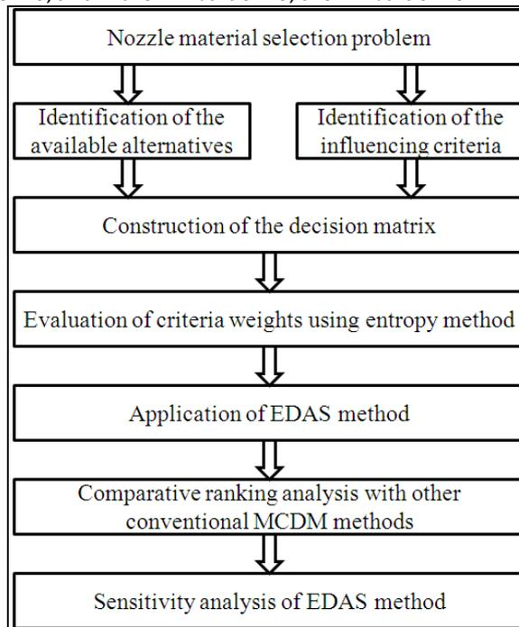
Figure 3. Steps of EDAS method for 3D printer nozzle material selection problem
