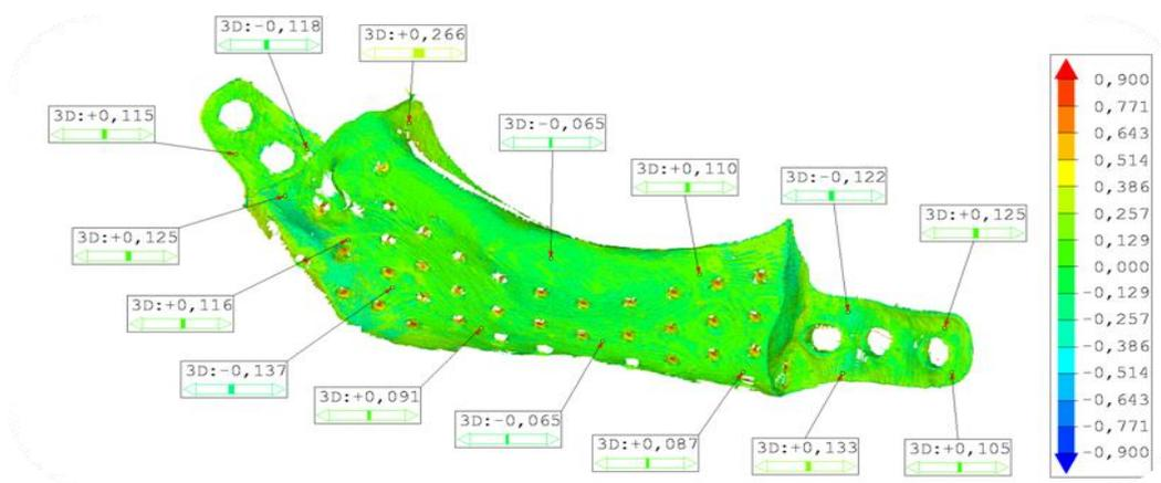
**Figure 5.** Generated map of deviations for a model supplementing the loss of the mandible
