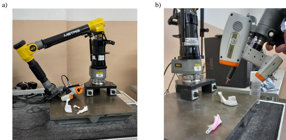
**Figure 4.** The stage of analysis of the accuracy of the models: (a) articulated arm with the MMD $\times$ 100 laser head; (b) measuring process
