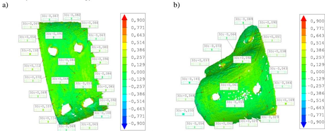
**Figure 6.** Generated maps of deviations for a resection template: (a) no.1; (b) no.2
