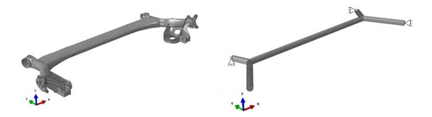
Figure 4. Industrial model and simplified beam model
