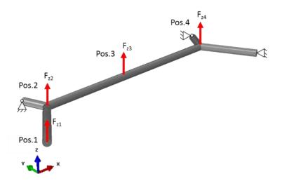
Figure 5. Boundary conditions and loading positions
